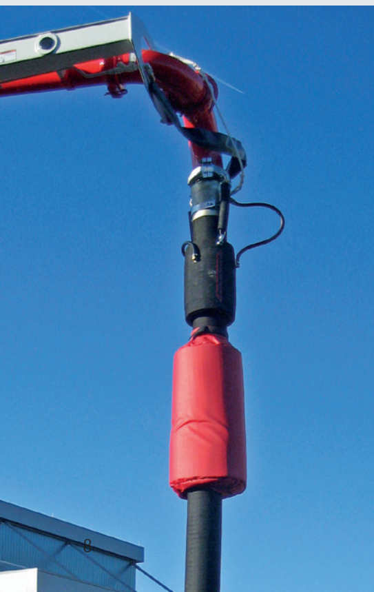
The end hose squeeze valve (EQV) closes securely and stops the flow of concrete
