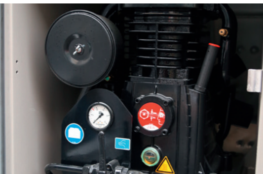
The compressor provides compressed air for various applications, e.g. cleaning
