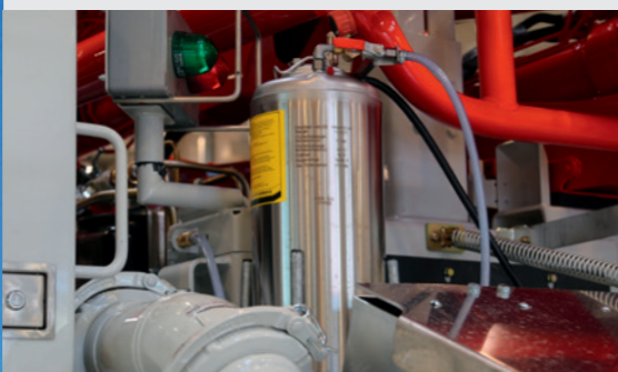
Spray tank with compressed air connection for easy cleaning of the hopper by moistening with release agent beforehand
