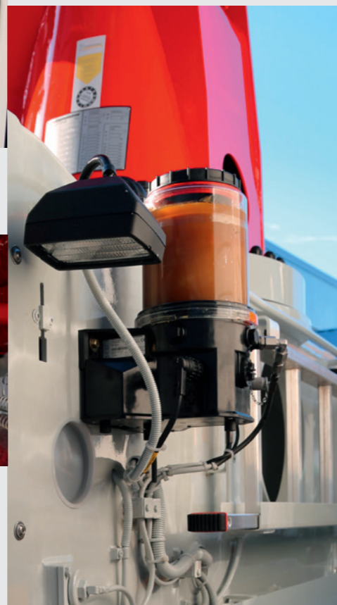
The central grease lubrication system on the boom reduces the time for daily maintenance
